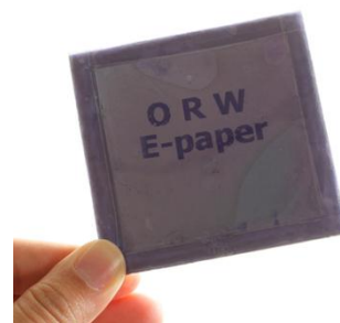
Optically rewritable e-paper enables writing, storing and rewriting information using light sources
